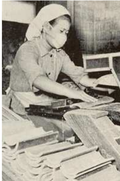
(2) After selection and rough cutting, pieces are formed using circular saw.
