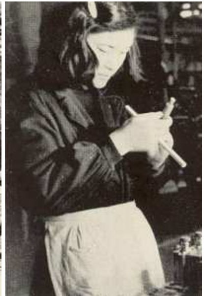
(9) Inspection: Checking thickness with micrometer.
