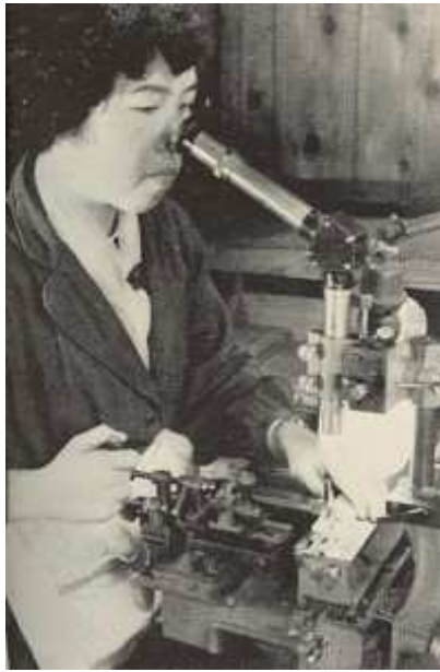
(13) In some rules, there is an index line on the back of the rule. Since accuracy is required, a line curving machine with microscope is used.
