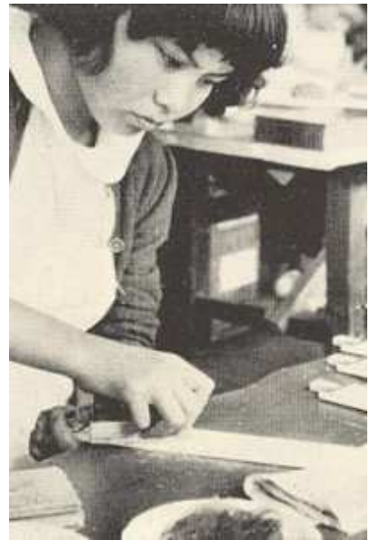
(12) Finish: After red markers are put in, and after inspection, the surfaces get polished.
