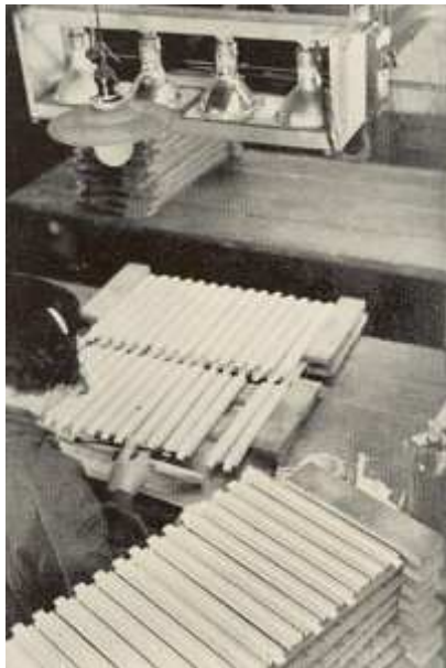
(10) Making grooves: It requires great attention since this is one of the areas on which accuracy of the slide rule depend.
