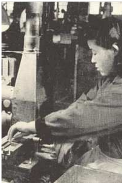
(4) After gluing two or four pieces together, a flat surface is milled out using this machine.
