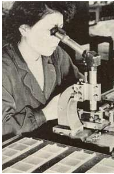
(14) Cursor line is created by first coating surface of cursor glass with wax and drawing a thin line and finally etching the glass.
